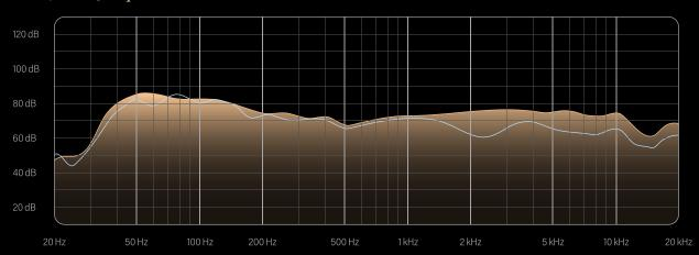
Pegasus Pro 0° on-axis & 90° off-axis comparison, boom pole fully extended, mic height 1.7 meters, mic distance from speaker 3 meters, volume set low.
