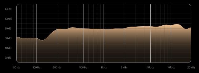
$Eros\,Pro\,flush\,mount\,1\,meter\,@2.83\,volts, full\,range, mounted\,in\,1x1m\,plaster, 1/6\,octave\,smoothing.$
